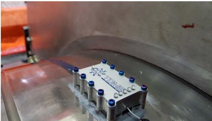
Figure 3 – Telemetry module attached to rotor surface.
