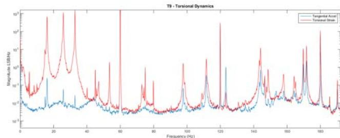
Figure 5 – Spectral plot of large steam turbine shaft torsional vibration, including both torsional strain and shaft surface tangential acceleration
