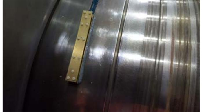
Figure 1 – On-rotor antenna configuration
