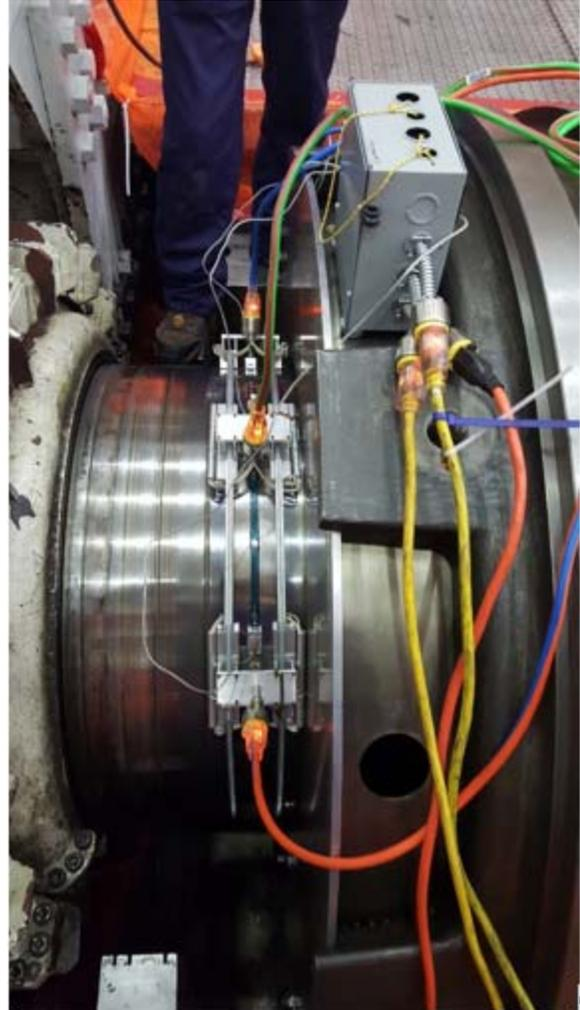
Figure 4 – Installation of two antennas and telemetry module on a 900mm diameter generator input shaft
