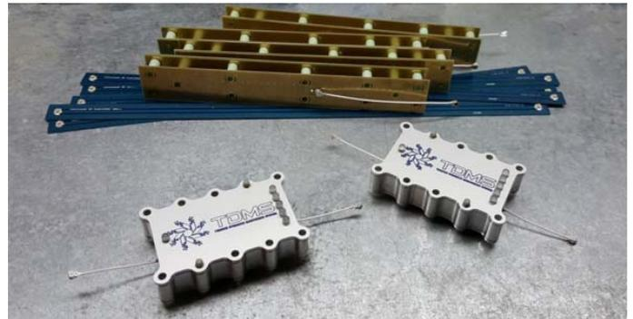
Figure 2 – Telemetry modules, waveguides, and antenna components.
