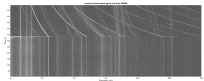
Figure 6 – Spectrogram of shaft torsional strain showing changes in frequency as a function of shaft speed following a unit trip
