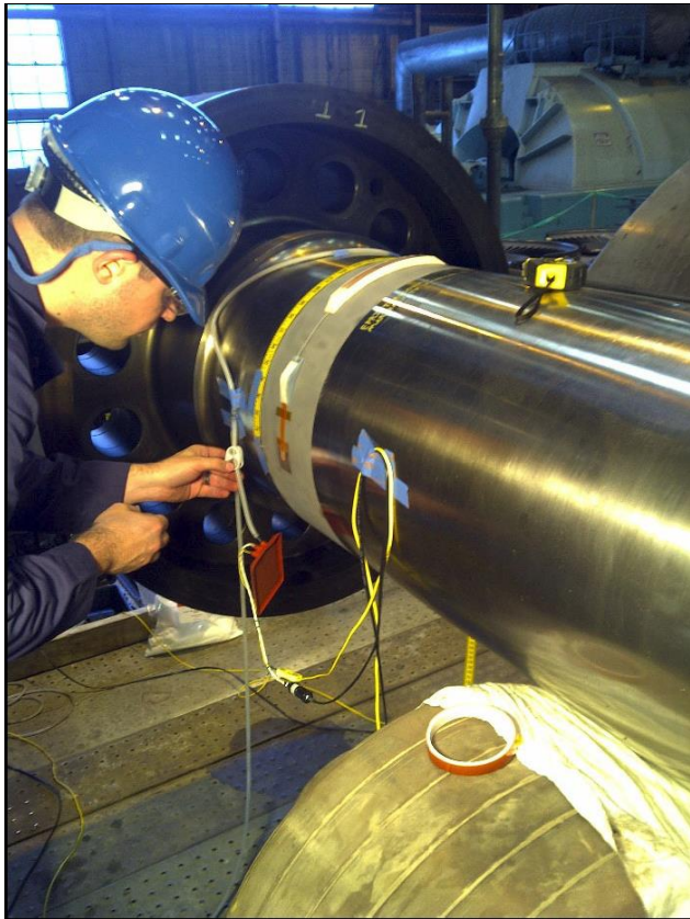
Figure 2. Prototype telemetry receiver components positioned on lightly abraded shaft section prior to epoxy encapsulation
