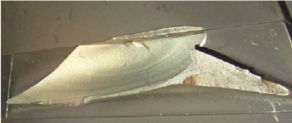
Failure of R0 Compressor Blade
